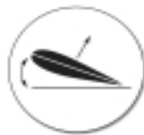
Chord Line runs thru center of wing
