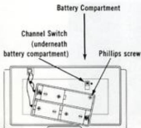
Remove Battery Cover Plate and install four batteries, following diagram. Replace Cover Plate with slot facing front of PONG Control Unit.
