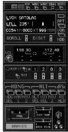
Here is a radio stack with a GPS, a NavCom radio that sends data to an HSI, and retractable gear as well. The aileron and rudder trim for fine-tuning the airplane are to the left of the gear handle.
