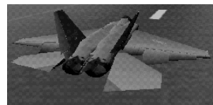
This modified F-22 not only shows stabilator/elevator roll differential (see its horizontal stab), but also aileron with elevator deflection to sustain high maneuverability. Flaps are in take-off position
