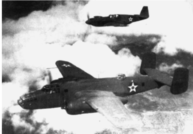
B-25D in formation with an A-36. The A-36 Apache was the early variant of the P-51 Mustang. Equipped with an Allison engine, the A-36 was used as a dive bomber/attack craft in Italy. Later, a British Merlin engine was mated to the airframe, creating the P-51B Mustang. (Courtesy Foto Consortium)
