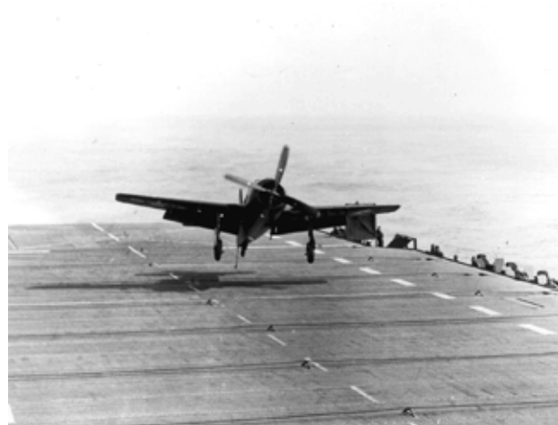
A Bearcat trapping aboard an Essex class carrier. Grumman stuffed the largest engine into the smallest, lightest airframe possible to create a plane so powerful it had no peer. (Courtesy National Air & Space Museum, Smithsonian Institution)
