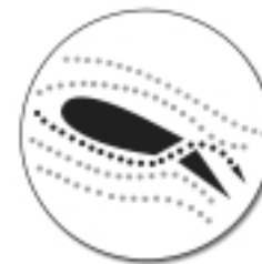
The air flowing through the slot between the wing and the flap helps keep the overall flow attached at very high angles of attack.
